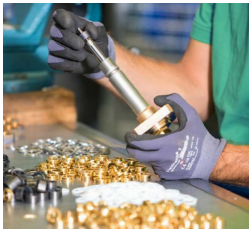
Careful assembly of the valve components
